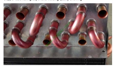
Aluminum fin drawing and expanding on copper tube, 100% wrapped the copper tube
